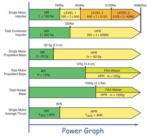
Take the black-powder D motor again. It has 21.1 grams of propellant mass. It would take only six of these to exceed the FAA propellant mass limits and require a waiver even though the impulse is only 102 newton-seconds. So there is more than one way to exceed the limits.
